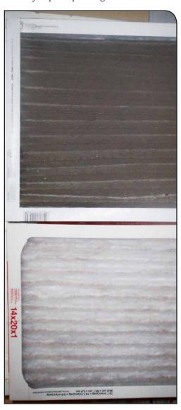
Compare to the new filter on the bottom to the filter installed 3 months ago. The photo does not show all the cob webs and dust bunnies that it holds.
